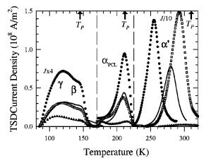
FIG. 4. TSDC spectra for the block copolymers and the PCL homopolymer: ( $\bullet$ ) PCL, ( $\triangle$ ) S<sub>57</sub>B<sub>27</sub>C<sub>16</sub>, ( $\Box$ ) S<sub>35</sub>B<sub>15</sub>C<sub>50</sub>, (line) S<sub>09</sub>B<sub>14</sub>C<sub>77</sub>. The polarization temperatures are indicated by arrows.
