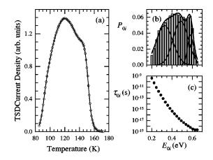
FIG. 5. Results of the DSA for the secondary relaxations in the homopolymer poly( $\epsilon$ -caprolactone): (a) experimental data and fitted profile; (b) energy histogram showing the contribution to the total polarization of each Debye process; (c) variation of the preexponential factor with the energy bin value for the Debye processes whose sum best describe the experimental profile.
