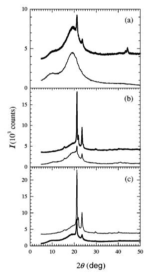
FIG. 3. WAXS spectra for the three block copolymers studied, in original conditions (thin line) and after annealing (thick line): (a)  $S_{57}B_{27}C_{16}$ , (b)  $S_{35}B_{15}C_{50}$ , (c)  $S_{09}B_{14}C_{77}$ .
