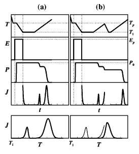
FIG. 1. Experimental protocol for the TSDC measurements with the variation of the temperature T, the applied field E, the polarization acquired by the sample P, and the depolarization current density  $J_D$ . (a) standard polarization procedure (b) peak cleaning procedure.
