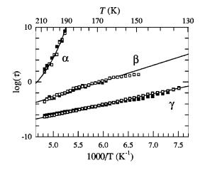
FIG. 10. Relaxation plot,  $\log_{10}(\tau) = f(10^3/T)$ , for the triblock copolymer S<sub>35</sub>B<sub>15</sub>C<sub>50</sub>: (filled squares) original material, (empty squares) annealed sample. The lines are the fitting of the experimental points to VTF ( $\alpha$  relaxation) or Arrhenius relaxation times ( $\gamma$  and  $\beta$  modes).
