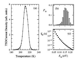
FIG. 6. Results of the SADSA for the  $\alpha$  relaxation in the block copolymer S<sub>09</sub>B<sub>14</sub>C<sub>77</sub>: (a) experimental data and fitted profile; (b) energy histogram showing the contribution to the total polarization of each Debye process; (c) variation of the preexponential factor with the energy bin value,  $T_0 = 157.5$  K.
