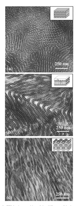
FIG. 2. TEM micrographies of the different triblock copolymer morphologies studied: (a)  $S_{57}B_{27}C_{16}$ , (b)  $S_{35}B_{15}C_{50}$ , (c)  $S_{09}B_{14}C_{77}$ . On the upper right corner is a schematic drawing of the microstructures observed.
