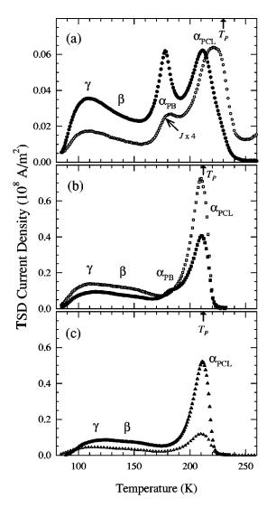
FIG. 8. TSDC spectra (T < 260 K) for the original (filled symbols) and annealed (empty symbols) block copolymers. (a)  $S_{57}B_{27}C_{16}$ , (b)  $S_{35}B_{15}C_{50}$ , (c)  $S_{09}B_{14}C_{77}$ . The polarization temperature is indicated by arrows.
