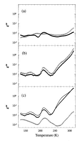
FIG. 9. Dielectric absorption spectra for original (filled symbols) and annealed (empty symbols) block copolymers. (a)  $S_{57}B_{27}C_{16}$ , (b)  $S_{35}B_{15}C_{50}$ , (c)  $S_{09}B_{14}C_{77}$ . The continuous line represents the homopolymer PCL<sup>93</sup>.
