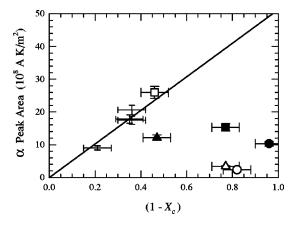
FIG. 7. Comparison of the amount of amorphous phase detected dielectrically, and the amorphous phase detected by WAXS,  $\alpha$  peak area vs  $(1-X_c)$ , for all the block copolymers and the PCL homopolymers. The filled symbols represent the original and the empty ones the annealed copolymers. + PCL homopolymers, ( $\bigcirc$ ) S<sub>57</sub>B<sub>27</sub>C<sub>16</sub>, ( $\square$ ) S<sub>35</sub>B<sub>15</sub>C<sub>50</sub>, ( $\triangle$ ) S<sub>09</sub>B<sub>14</sub>C<sub>77</sub>.
